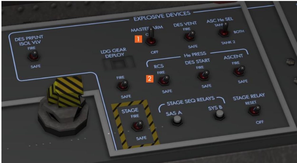
Figure 6.2.1.2 – RCS pressurization on the EDS
